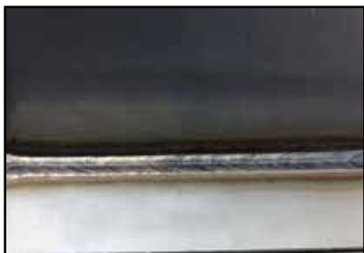
■ CrNi sarokvarrat PB | 1,0 mm POWER.ARC
