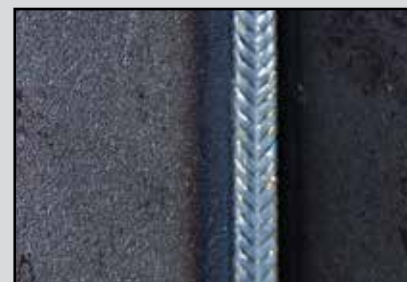
■ Acélsarokvarrat PF | 5,0 mm POWER.PULS (duplaimpulzus)
